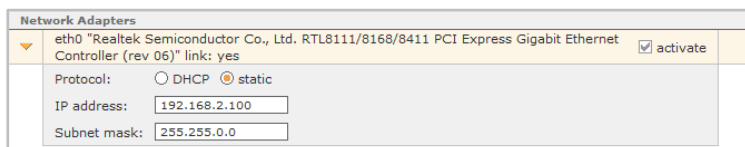
Figure 33 – Example of eth0's static configuration
